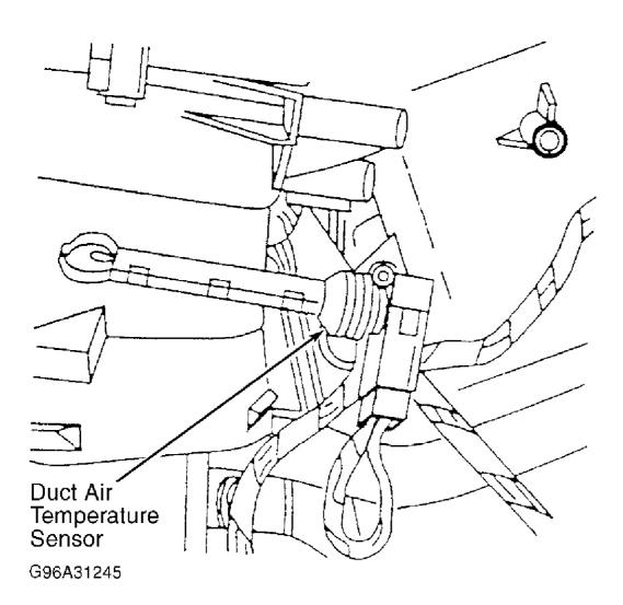
Fig. 5: Removing Duct Air Temperature Sensor
