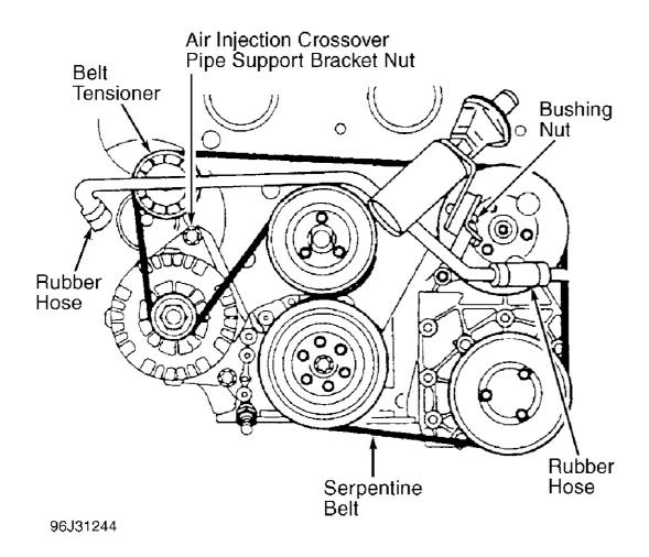
Fig. 4: Serpentine Belt Routing Courtesy of GENERAL MOTORS CORP.
