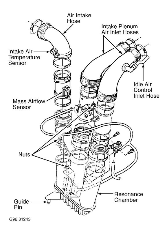
Fig. 3: Removing Resonance Chamber Courtesy of GENERAL MOTORS CORP.
