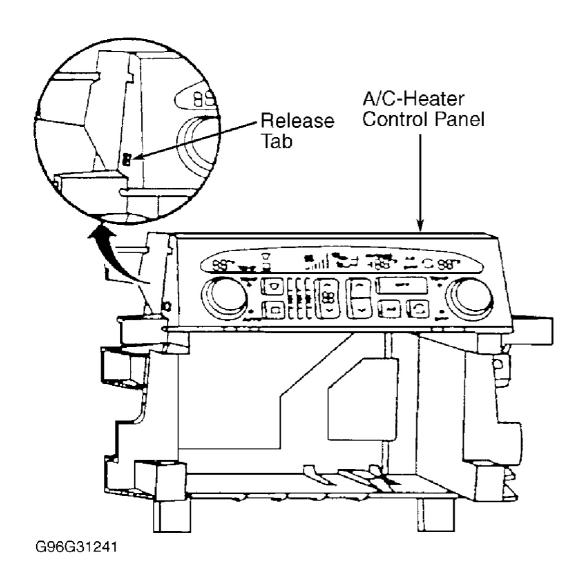
Fig. 1: Removing A/C-Heater Control Panel Courtesy of GENERAL MOTORS CORP.
