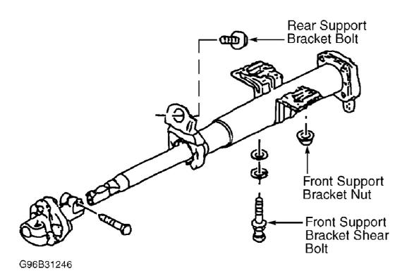
Fig. 6: Removing Steering Column
