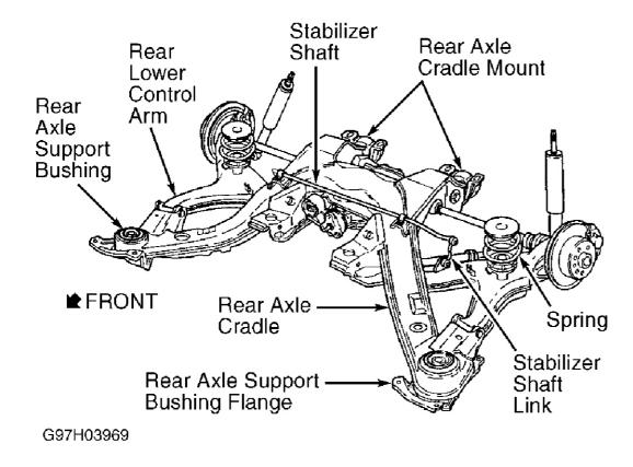
Fig. 1: Identifying Rear Suspension Assembly Components Courtesy of GENERAL MOTORS CORP.
