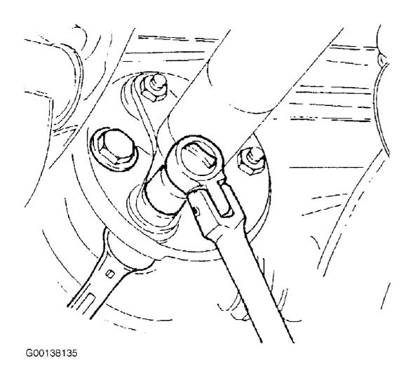
Fig. 3: Removing & Installing Coupling Bolts Courtesy of GENERAL MOTORS CORP.
