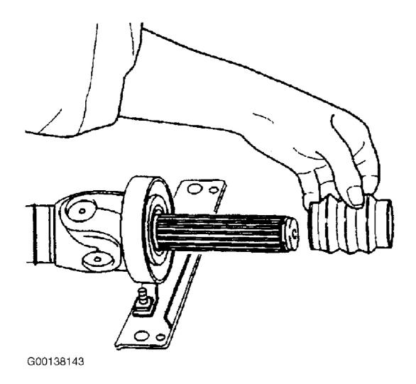
Fig. 13: Installing Boot
