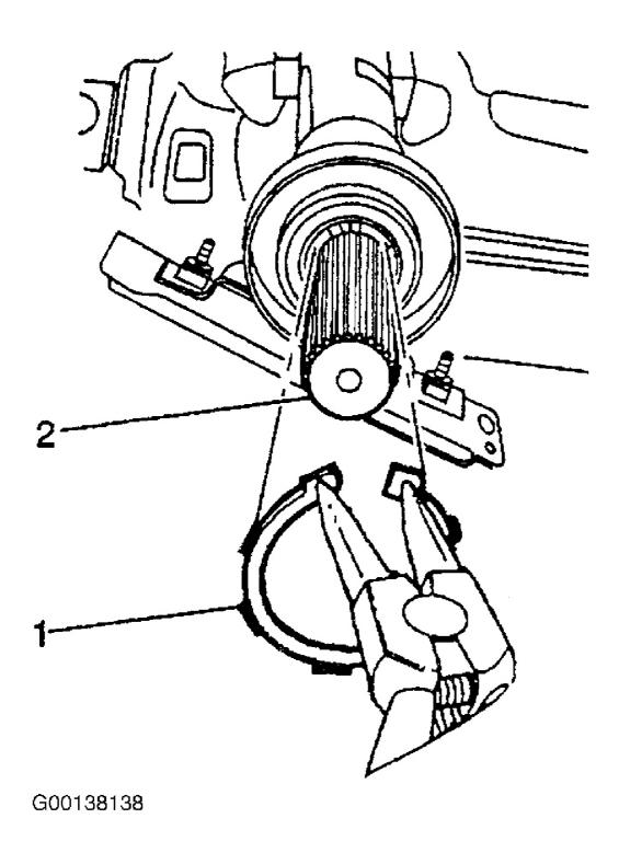
Fig. 6: Removing & Installing Front Retaining Ring From Journal Courtesy of GENERAL MOTORS CORP.
