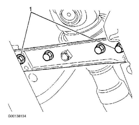
Fig. 2: Removing & Installing Bolts From Driveshaft Courtesy of GENERAL MOTORS CORP.
