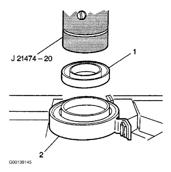
Fig. 11: Assembling Center Bearing Courtesy of GENERAL MOTORS CORP.
