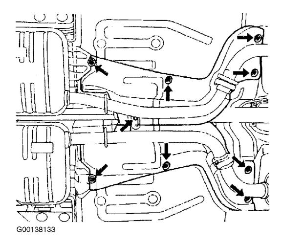
Fig. 1: Removing & Installing Heatshields & Nuts Courtesy of GENERAL MOTORS CORP.
