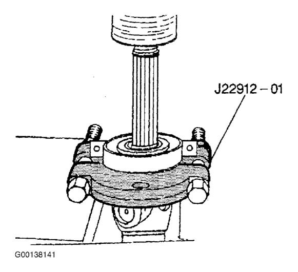
Fig. 9: Pressing Bearing Off Shaft Courtesy of GENERAL MOTORS CORP.
