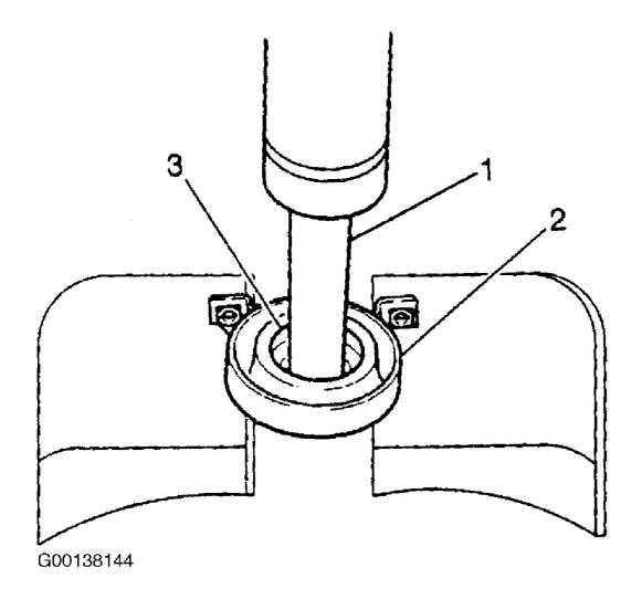
Fig. 10: Disassembling Center Bearing Courtesy of GENERAL MOTORS CORP.
