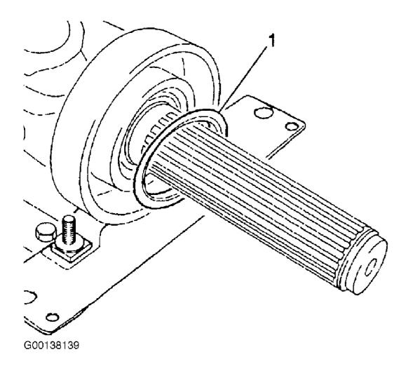
Fig. 7: Removing & Installing Slinger
