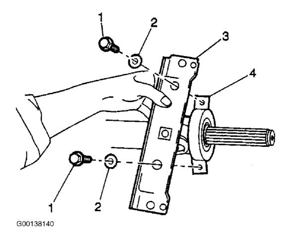
Fig. 8: Removing & Installing Bracket, Insulator, Bolts & Washers Courtesy of GENERAL MOTORS CORP.
