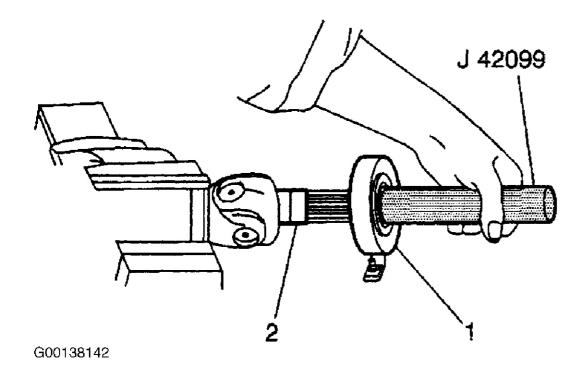
Fig. 12: Installing Bearing Onto Driveshaft Courtesy of GENERAL MOTORS CORP.
