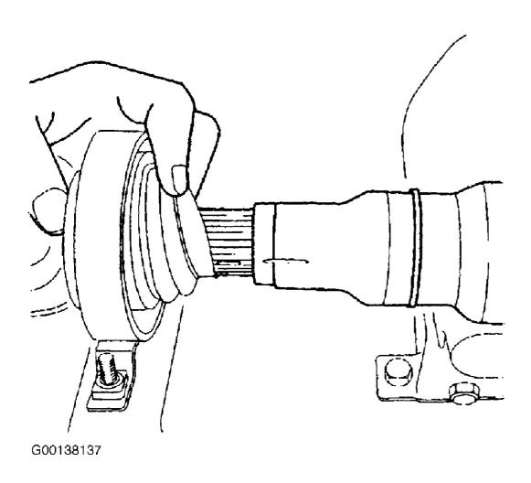
Fig. 5: Marking & Separating Propeller Shafts Courtesy of GENERAL MOTORS CORP.
