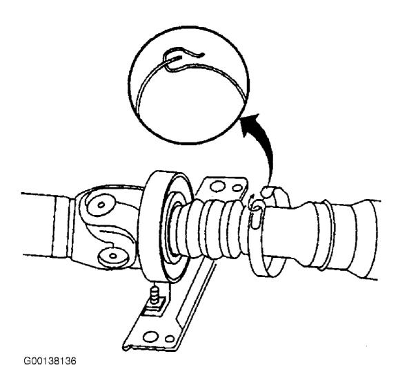
Fig. 4: Removing & Installing Propeller Shaft Slip Yoke Courtesy of GENERAL MOTORS CORP.
