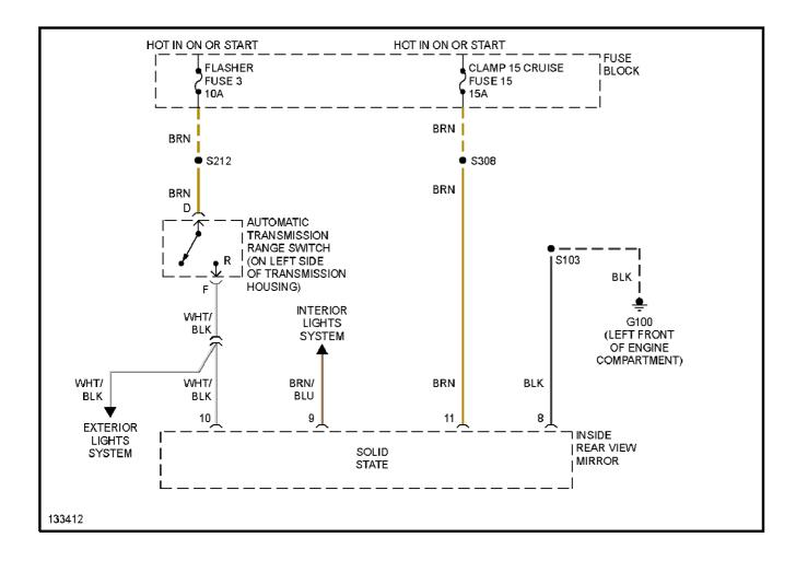
Fig. 2: Automatic Day/Night Mirror System Wiring Diagram (Catera)
